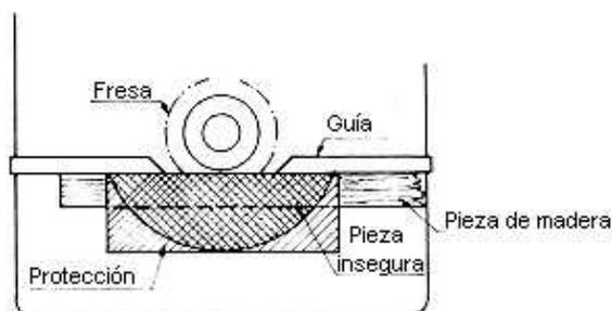
**Fig. 17: Esquema del cobertor de pantalla frontal (Fuente: Department of Labour, New Zealand)**
